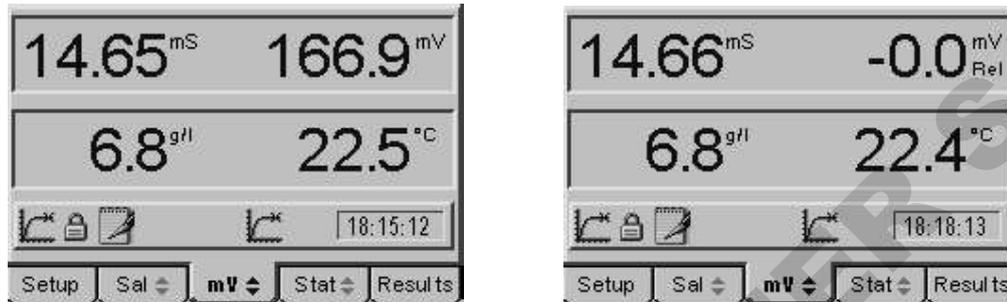
An absolute mV reading of 166.9mV is set to zero in Relative mV mode by pressing the CAL key
