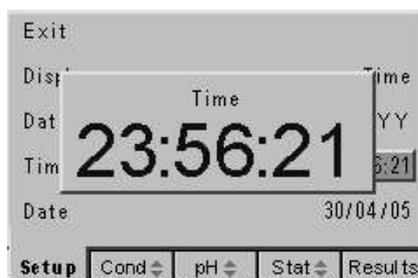
Data entry box for adjusting the time setting
