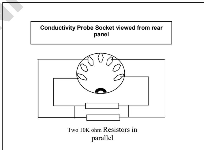
conductivity reading should be between 180 and 220 $\mu$ S depending on the last calibration or cell constant setting – if in doubt set the cell constant to 1.000 and re-check. If this functions correctly then any problem is most likely to be associated with the probe – if it fails to work correctly contact your local distributor or Jenway for service advice.
