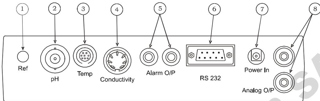
Rear Panel showing Input and Output Connectors
