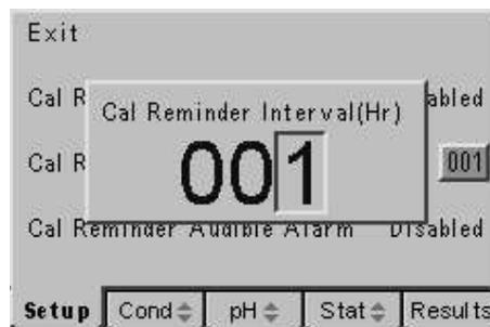
Data box for setting the Cal reminder Interval in Hours
