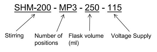
Note: Non-Stirring models are prefixed "HM-200" Number of Positions: 3 or 6 Flask volume size: 100ml, 250ml, 500ml, 1000ml Supply Voltage: Model numbers not suffixed "-115" = 230V a.c Please check the contents of your carton against the relevant product diagram. Applicable to all HM-200 Multi-position products.
