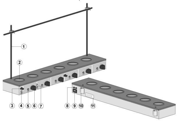
**7.2.2.** Switch on the mains electrical supply. Adjust the controller regulator knob in each position to the required setting.
