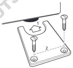
Ensure the unit is positioned correctly. From the sides of the unit, slide the feet brackets around
