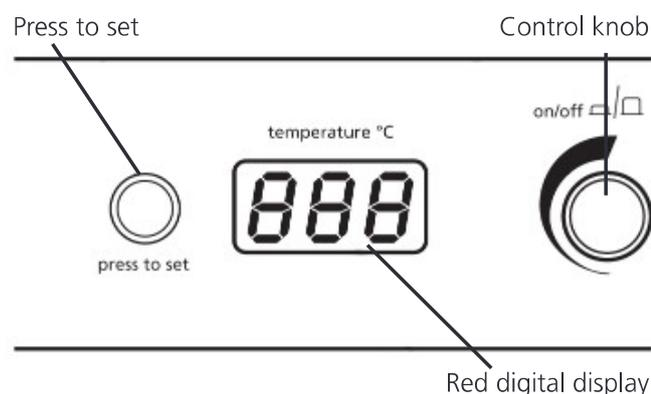
5. Release the "press to set" button. The incubator will then begin to heat to the set temperature. The actual temperature inside the chamber will be displayed on the screen.
