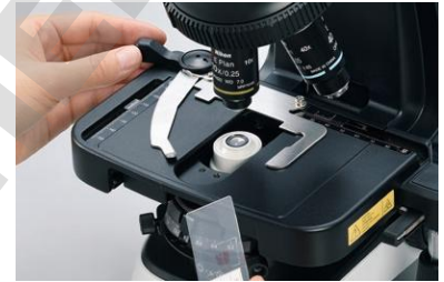
Easy-to-operate specimen holder
