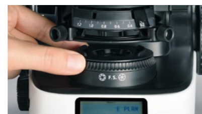
Turn the field diaphragm dial until the illumination range is circumscribed to the field of view.
