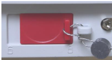
Locked with Wire Seal
