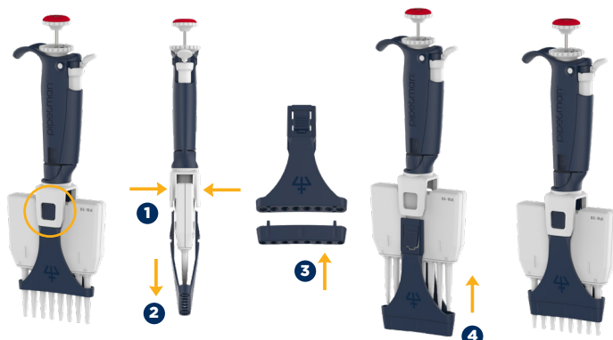
Figure 13 Fitting ejector adapter on multichannel models
