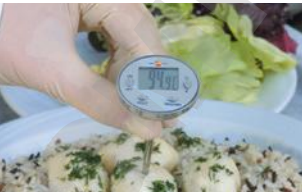
For temperature spot-check measurements in food production
