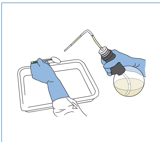
Figure 26. Flushing filter with solvent filtering dispenser.
