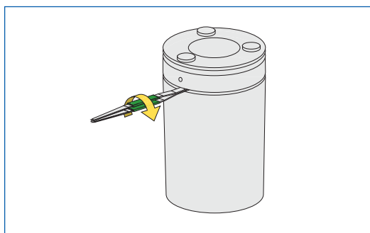
Figure 30. Remove 47 mm filter holder assembly from vacuum filtration flask.
