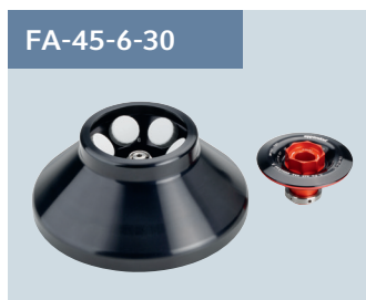
FA-45-6-30 6 × 50 mL conical tube rotor with aerosol-tight QuickLock lid for tubes from 5–50 mL. Max. speed 16,639 × g (11,000 rpm).
