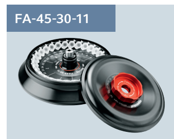
FA-45-30-11 30 × 1.5/2 mL micro tube rotor with aerosol-tight lid for safe centrifugation of hazardous samples. Max. speed 20,800 × g (14,000 rpm).
