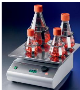
Orbital shaker with optional clamps and flasks
